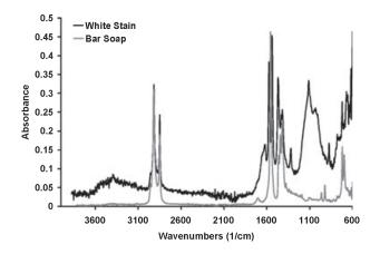
FIG. 4—FTIR spectra of  $(\blacksquare)$  the light sample and  $(\blacksquare)$  commercial bar soap.
