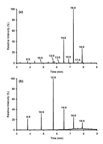
FIG. 6—Selected ion monitoring (SIM) chromatograms of m/z 87 for (a) the light sample and (b) commercial bar soap.
