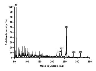
FIG. 5—Time-averaged (1.5–2.6 min) chemical ionization mass spectrum obtained during direct insertion probe analysis of the light sample.
