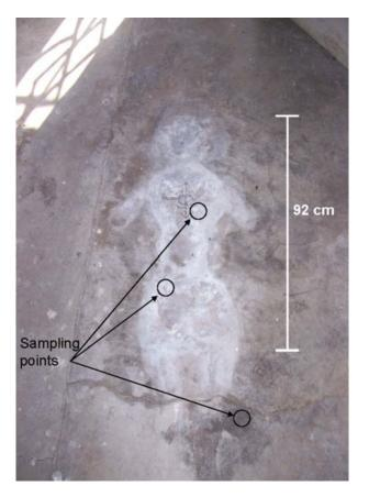
FIG. 1—Photograph of the questioned stain on the concrete floor showing the light area surrounded by a darker border.
